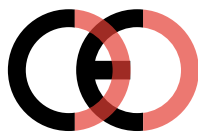
False CE Mark (too close)
