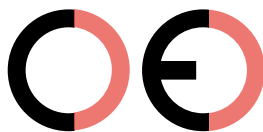
False CE Mark (too far)
